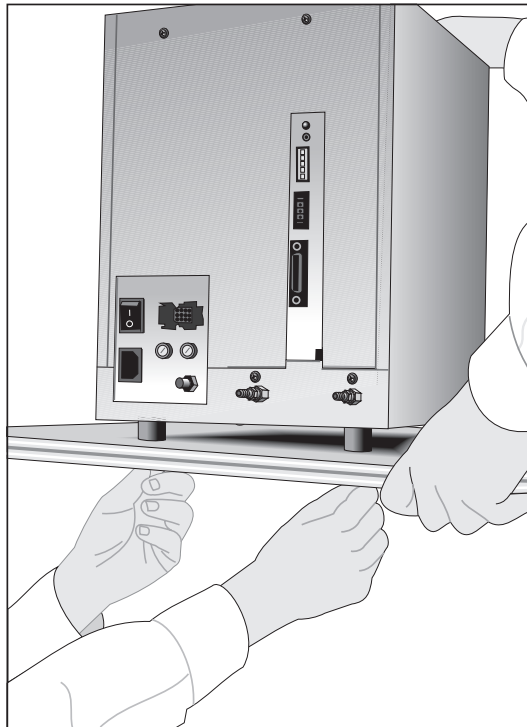
Figure 2.2 Removing the Plywood Board
